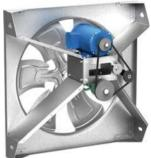
tensioner will adjust tension as the belt wears, easily doubling the life of the belt while maximizing the life of the fan and motor. Fan efficiency is also improved as proper belt tension minimizes drive loss. Model BAER is available in exhaust configurations with propeller diameters from 24 to 36 inches, and performance capabilities from 300 to 33,000 cfm and up to 3.3 in. wg.
